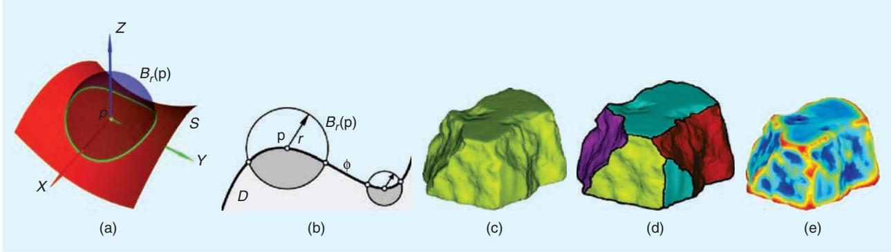
**[FIG14]** These images demonstrate how the authors compute integral invariants (a) and (b) [see (5) and (6)] and associated text for details. (c) and (e) show how a raw digitized fragment (c) is segmented, (d) compactly represented in terms of one exemplar invariant feature: (e) surface sharpness. These invariant features are further compacted and then used for fracture surface and break curve matching. (Used with permission from [11].)
