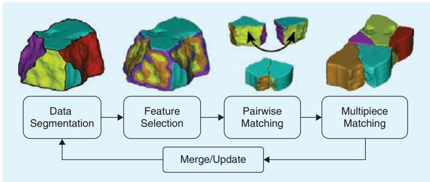
**[FIG4]** The generic process for object reconstruction. It consists of four steps (from left to right): 1) classify the boundaries of interest for matching, 2) compute a shape model for these boundaries in terms of features, 3) search for correct pairwise matches of the computed features and 4) implement a merge and update procedure that merges pairwise matches into larger multipiece configurations. (Used with permission from [11].)
