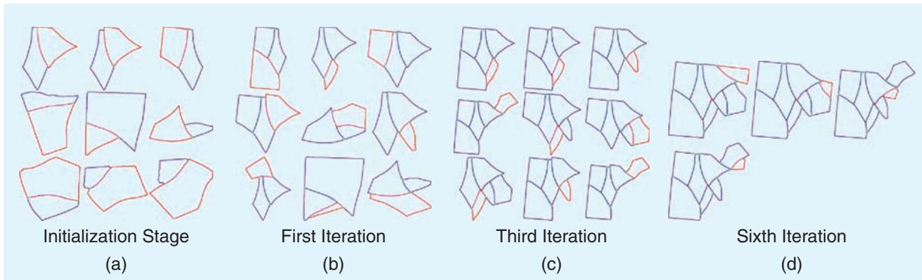
**[FIG8]** Nine fragment pairs, shown in (a), are chosen as different starting points for reconstructing a ceramic tile. The results of the best-global-first search for matching fragments are shown at iterations (b) 1, (c) 3, and (d) 6. (Used with permission from [1].)
