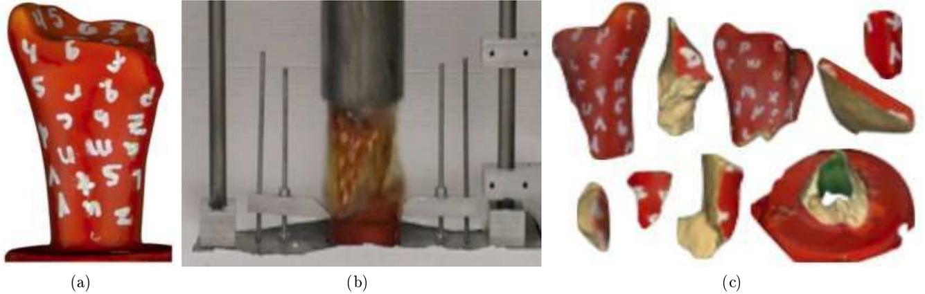
Figure 2: (a) Distal tibia replicas (3D laser scan shown, with photographic texture overlaid), machined from bone surrogate material, are marked to allow definitive post-fracture identification of the site of origins for each of the bone fragments. (b) A frame from a high-speed video of an impact event is shown here. A custom drop-tower is used to deliver a fracturing impact to the bone, embedded in a soft tissue simulant gelatin. (c) Bone fragments are laser scanned for virtual reconstruction.
