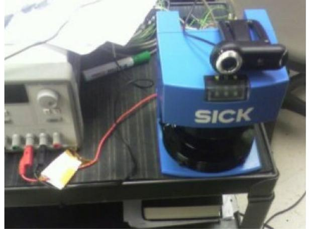
Figure 1. An image of a calibrated LIDAR-and-camera system consisting of a SICK LMS200 and an inexpensive commodity USB web-camera.
