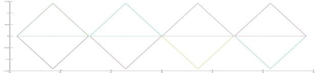
Figure 2. A top-down view of the 3D model used as the simulated calibration pattern. It consists of four adjacent boxes that touch at their corners.
