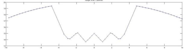
Figure 4. A plot of the sensed LIDAR depths observed from the simulated virtual calibration pattern from Figure XX. Depth measurements are divided into local linear segments by line-fitting and the calibration pattern corners are extracted.
