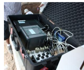
Figure 6: Permanently mounting the computers in a case simplified setup and made the connections more reliable
